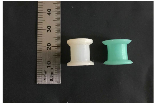
FIGURE 6 Comparative image of the 3D-printed silicone stent on the left and the commercially available stent on the right. Note the 1 mm increased length and rounded flanges of the 3D printed device.
