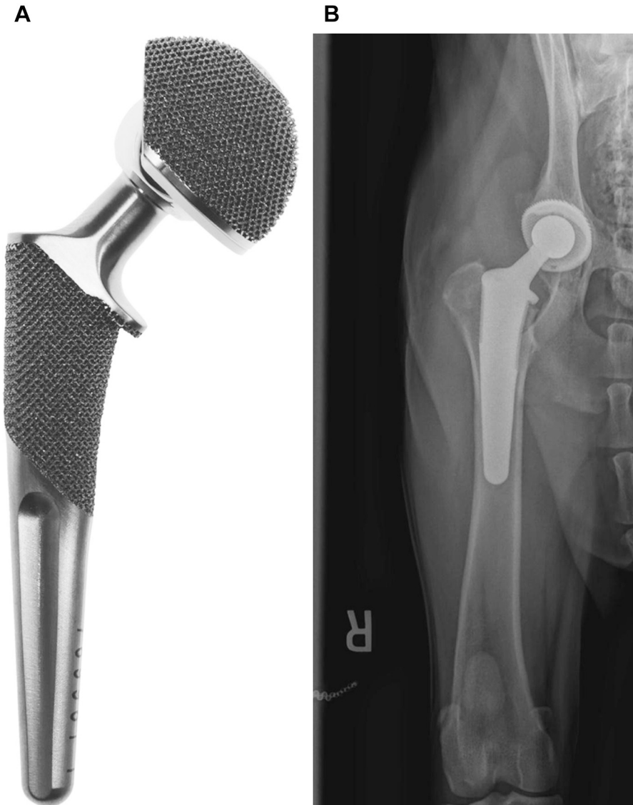
Fig. 4. BioMedtrix collared BFX stem and cup. (A) The collared BFX EBM titanium stem has a collar extended from the cranial aspect of the implant. The underside of this collar is porous to allow bone ingrowth. The collar is positioned at or just above the cortical bone edge of the neck cut and functions to potentially decrease the risk of subsidence. (B) A 3-month postoperative radiograph of a BFX collared stem in a 45 kg, 3-year-old German Shepherd dog. (Implant image Courtesy of BioMedtrix, LLC, Whippany, NJ.)
